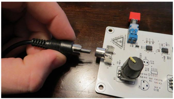
Plug other end of RCA cable into RCA Jack on controller.
