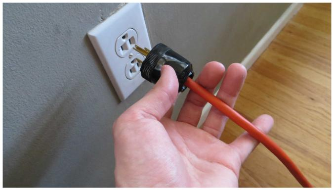
Plug Screamer into 120VAC outlet only. Must have be three prong type.
