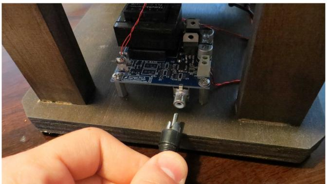
Plug RCA cable (not supplied) 6 feet or longer into RCA Jack on Screamer™Tesla Coil.
