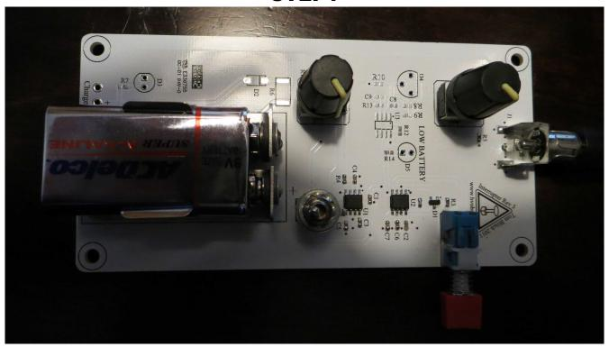
Insert fresh 9V battery into controller.
