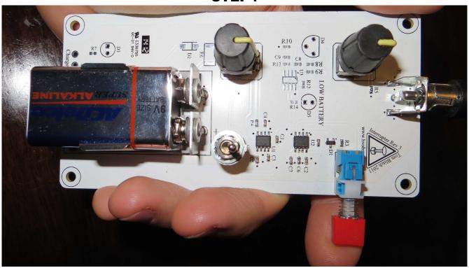
Rotate both knobs so they are both at midpoint (towards RCA jack)
